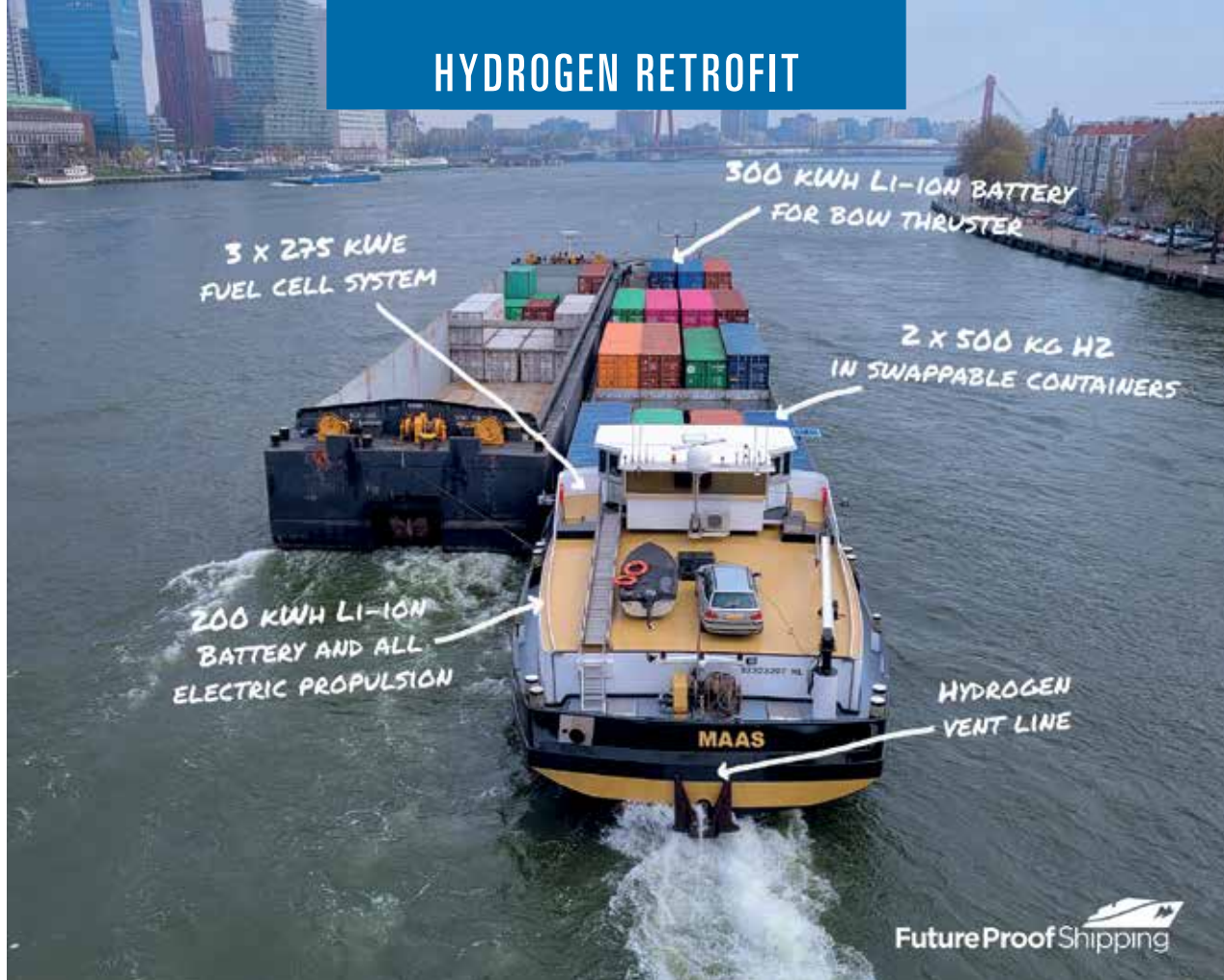
Location of the fuel cells, batteries and hydrogen system on board the FPS Maas.
