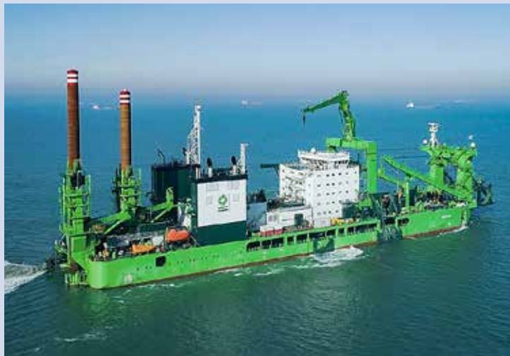
The Spartacus is the world's most powerful cutter suction dredger to date (photo Royal IHC).
