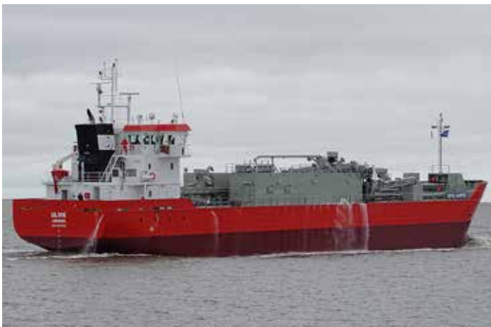
The pneumatic cement carrier Ulvik is the first in a series of four (photo F.J. Olinga).
