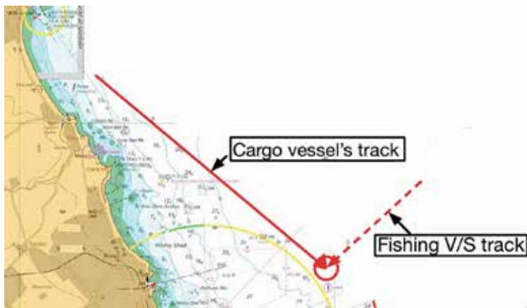
The tracks of the general cargo vessel and fishing vessel before they collided.
