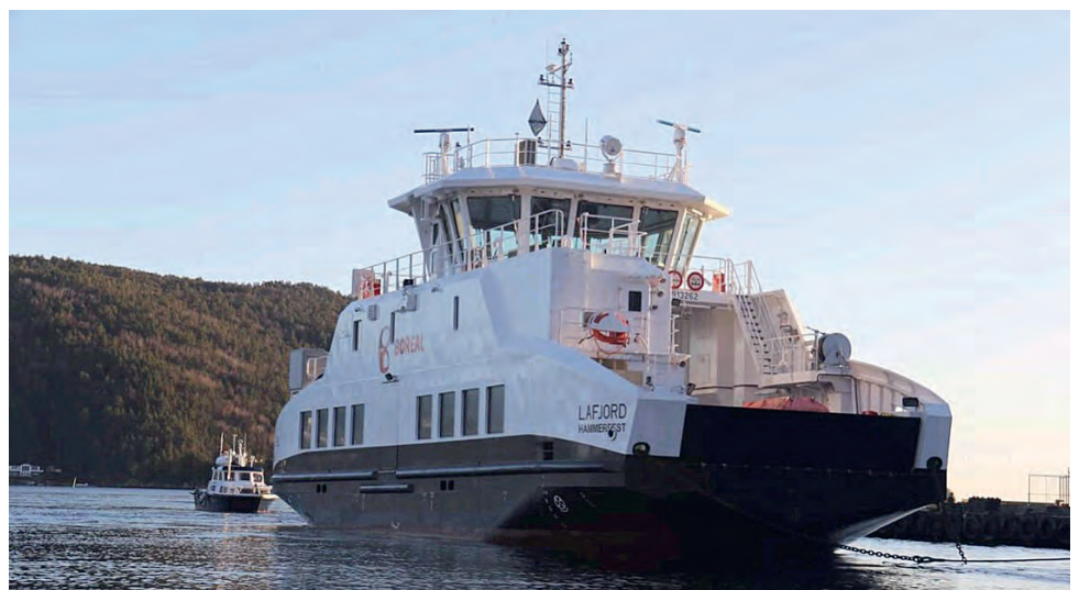
The fully electric double-ended shuttle ferry Lafjord .
