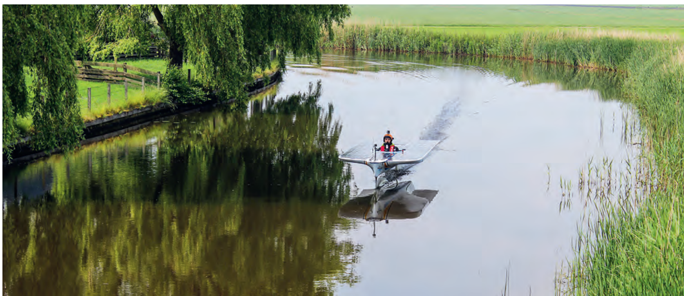
The TU Delft Solar Boat of 2016 illustrates how small the waves of a hydrofoil ship can be at 17 knots.
