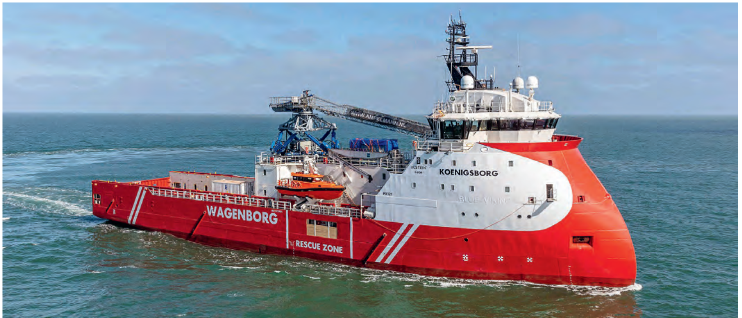
The Koenigsborg is a converted platform supply vessel, type Ulstein PX-121 (photo Flying Focus).
