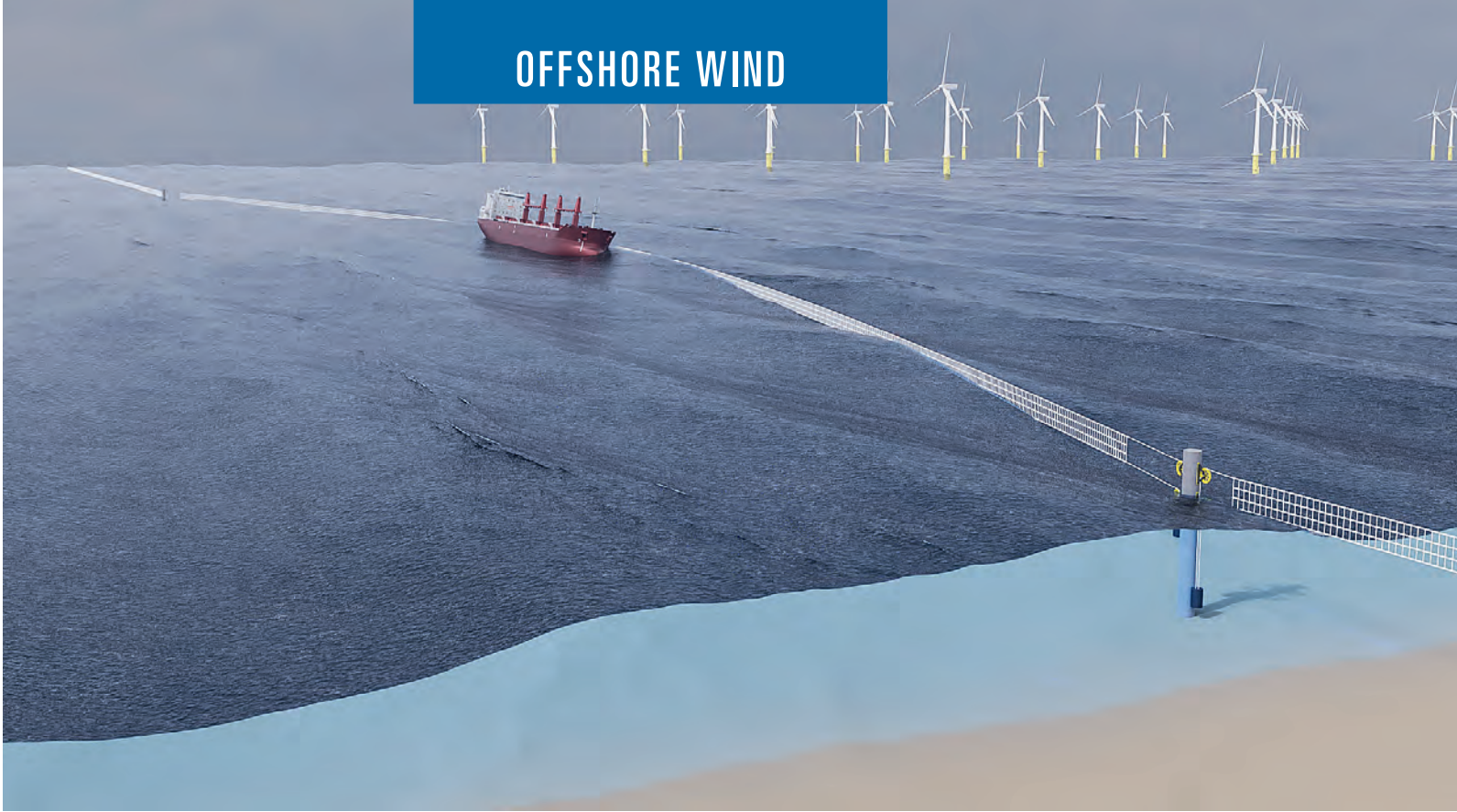
The third option is a pre-tensioned safety net.
