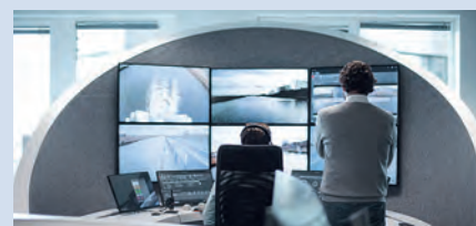
Seafar captains direct ships remotely from a control room and steer up to three ships at a time.
