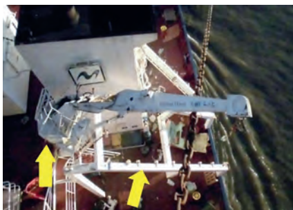
Stern crane and lifeboat torn off by large anchored vessel's anchor chain.
