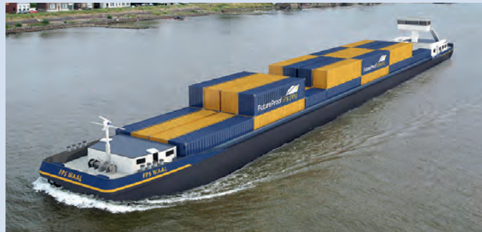
The retrofit of the FPS Waal will see the engine removed, and the zero-emission propulsion system including PEM fuel cells, hydrogen storage, battery packs and an electric drive train installed.
