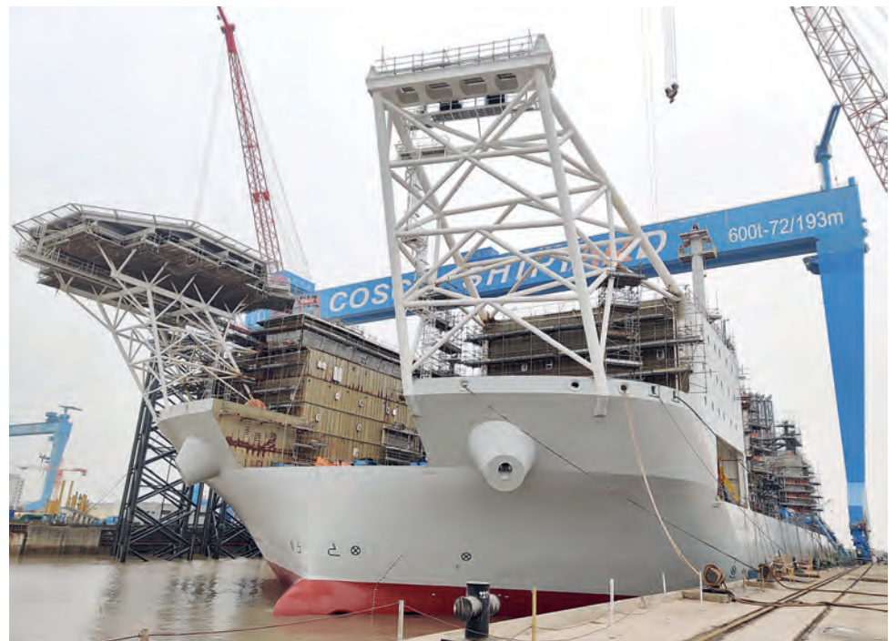
The offshore jack-up installation vessel Voltaire.
