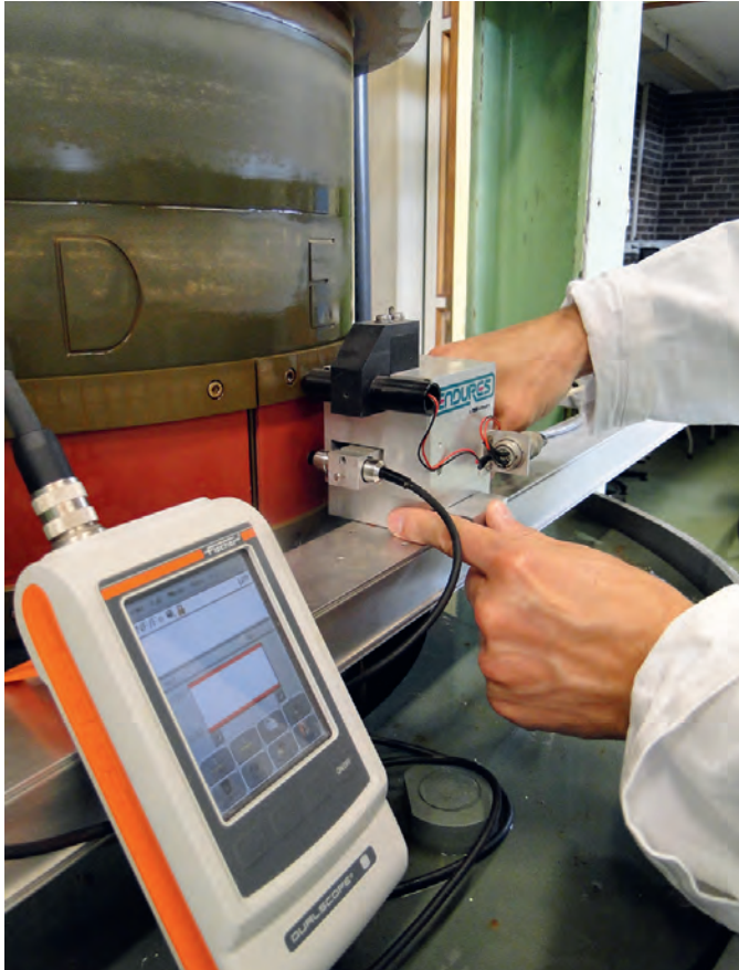
Polishing test on an antifouling coating.
