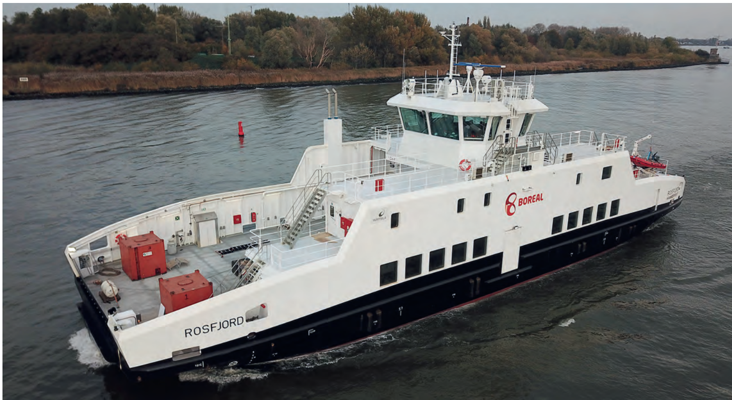
The fully electric double-ended shuttle ferry Rosfjord (photo A. Boer).
