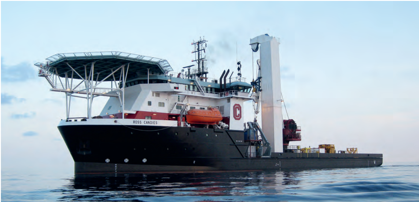
Offshore support vessel IMR (Inspection Maintenance and Repair) Ross Candies, Jones Act compliant, designed by Otto Candies Design Group, consisting of the author and a Polish design office (MMC). Built by Dakota Creek Industries, Anacortes, Washington State, in 2010. The 100-tonne deep-water deployment and recovery system (the mast on portside) was delivered by Huisman Equipment in Schiedam, the Netherlands. The ship won the Ship of the Year award in the US in 2010.
