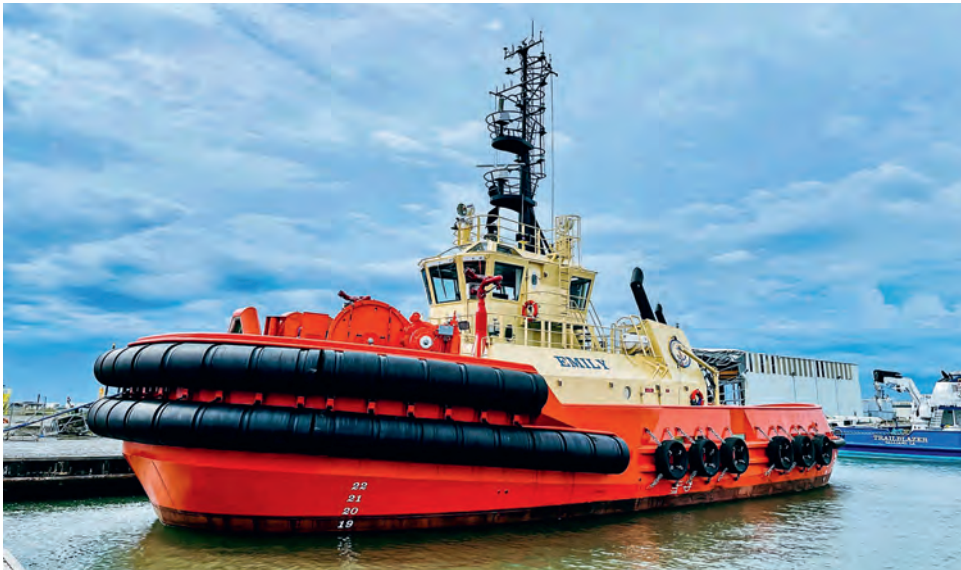
The Emily is one of four ASD Tugs 3212 built under Damen licence.
