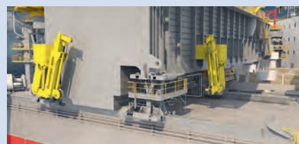
The Chela Twins cranes work at the well centre in pairs.
