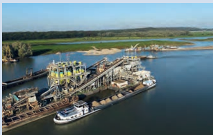
Dekker Group's floating sand plant can now use shore power to reduce emissions.
