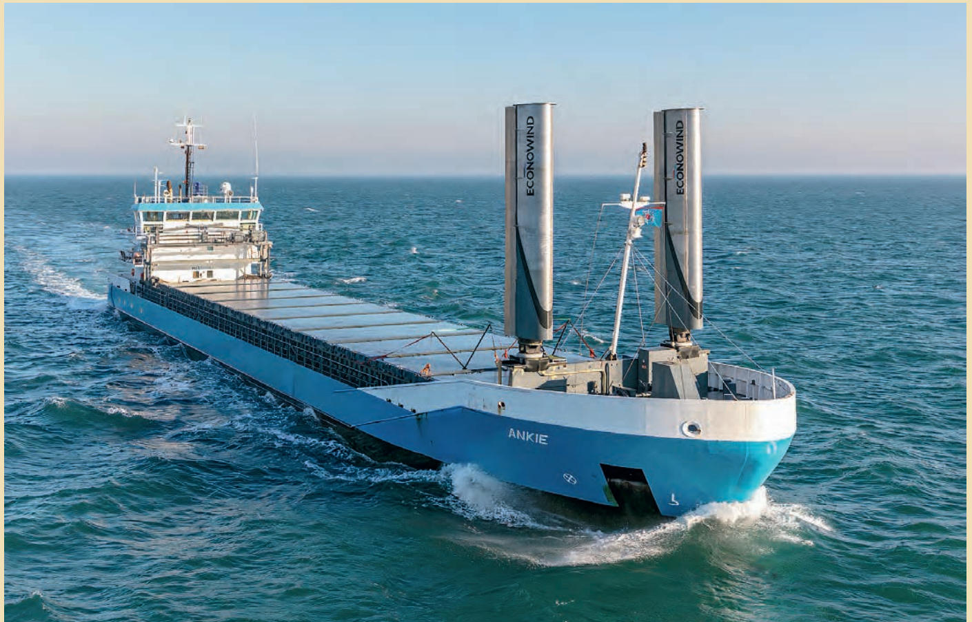
The first commercial installation of Econowind's Ventifoil system on Van Dam Shipping's Ankie.
