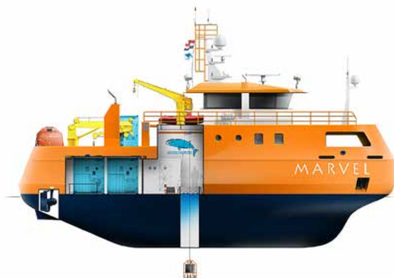
Side view of the MARVEL with a representation of the retractable azimuth thrusters, the moonpool and the 20 ft containers.
