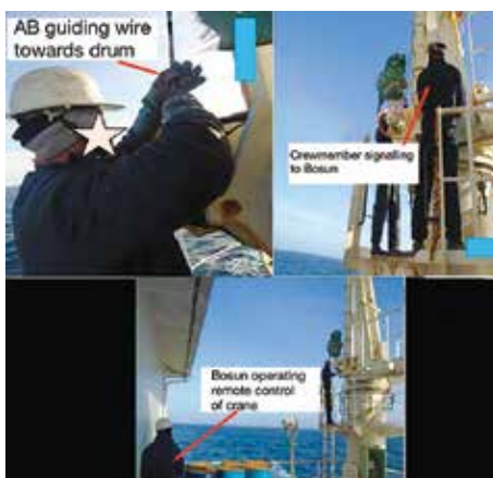
At one point, wire pinched the fingers of the crew member guiding it.
