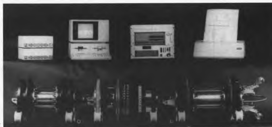
fig. 5: 16 in. RPIT with electronics to store, process, transfer and record data
