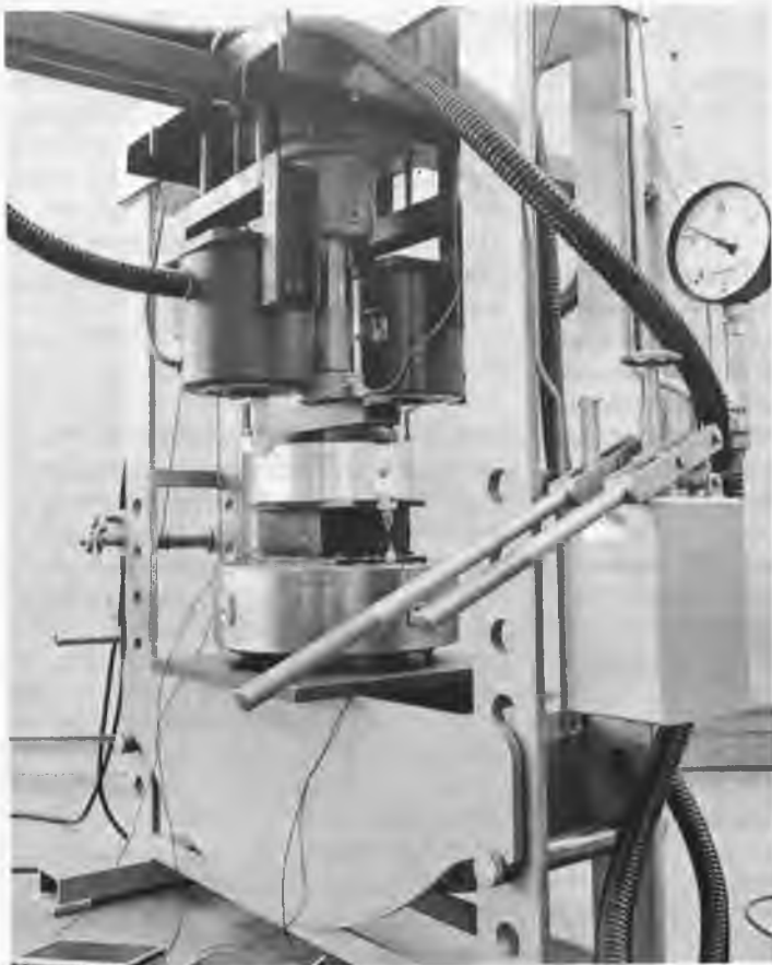
Fig. 4. Test rig with measurement configuration for T_{Fz,z} .
