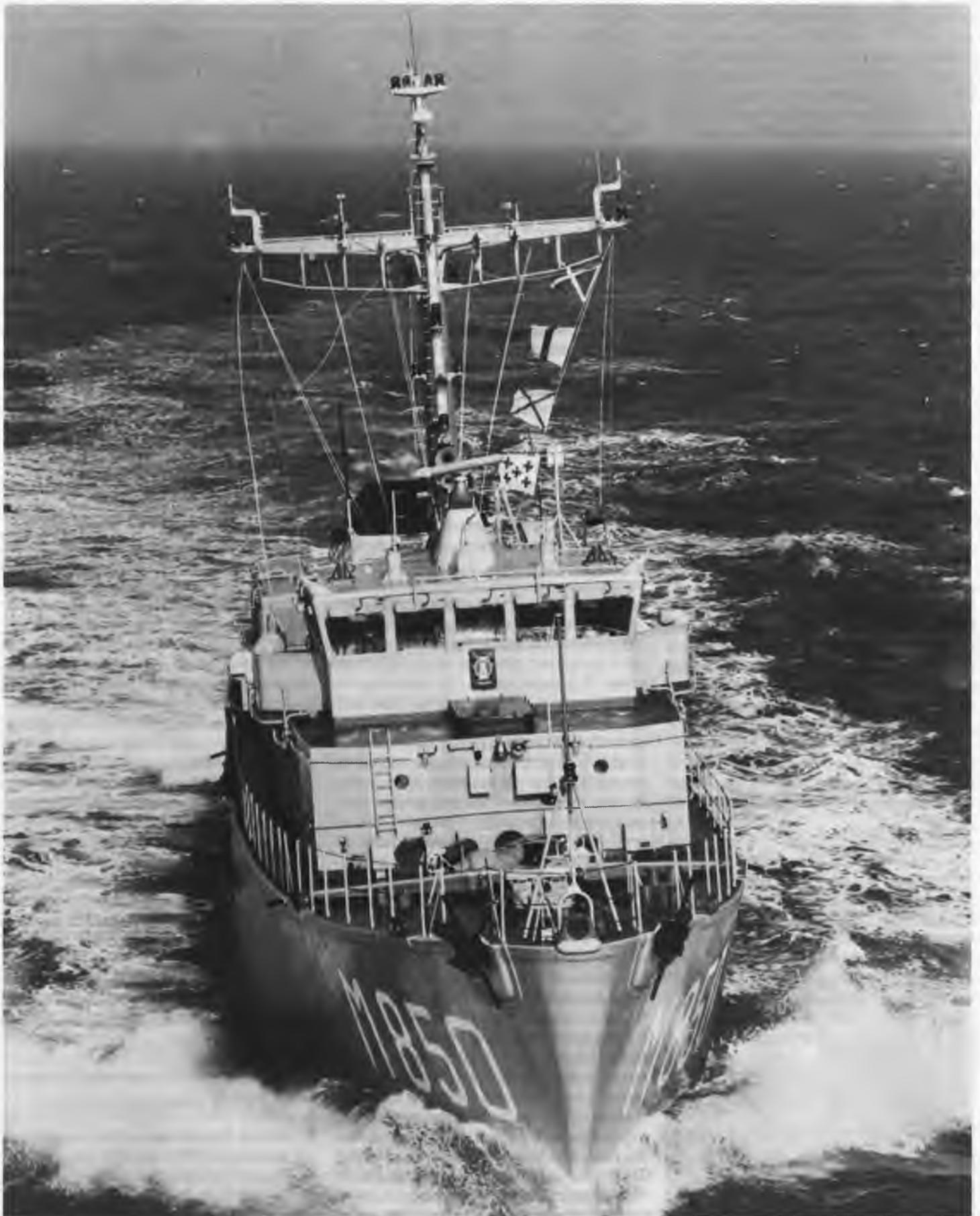
HNMS 'Alkmaar', the first of a series of 15 Tripartite mine-hunters commissioned on the 28 th of May 1983. The GRP-hulled ship is built by Van der Giessen-De Noord and powered by an A-RUB 215 dieselengine, 1400 kW built by Brons Industrie, good for a speed of 15 knots.
