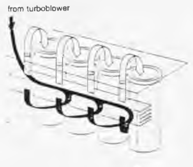
Fig. 10. Air ducting in the in-line engine frame.
