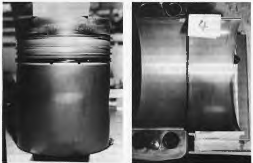
Fig. 15. Piston (left) and connecting rod bearing (right) after approx. 6000 hours of engine operation.
