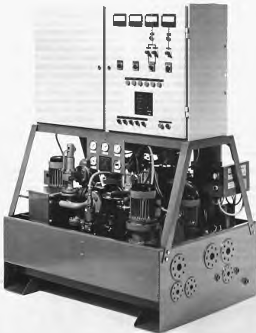
Fig. 1. The IMO on-line fuel oil conditioner.
