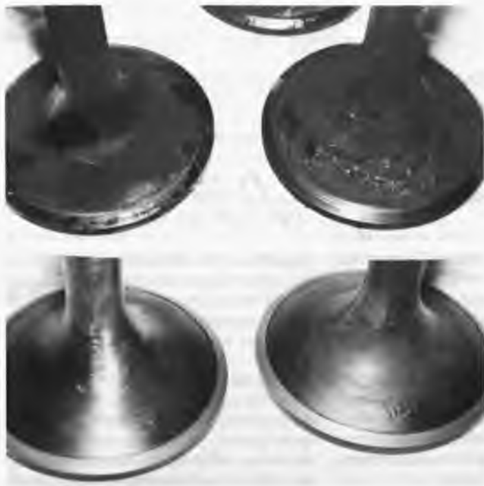
Inlet and outlet exhaust valves before and after cleaning. 7000 hrs. Bell Reliant.
