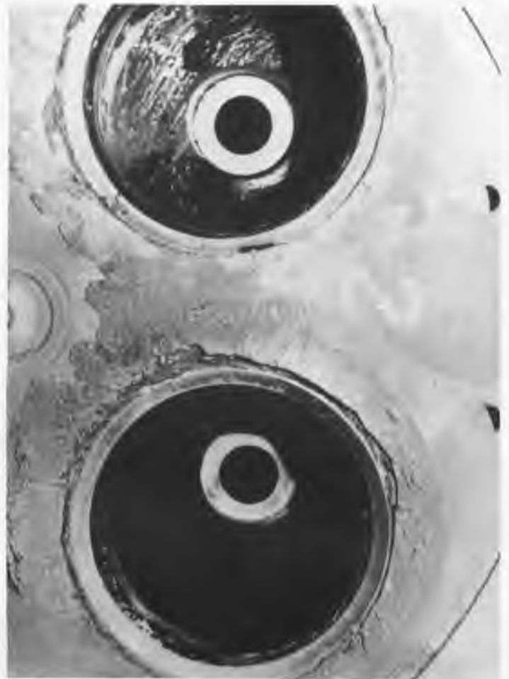
Fig. 3 Inlet port of Vasa 32 after 6400 h operation at low load. The port is entirely clean.
