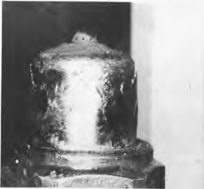
Fig. 2 Vasa 32 nozzle after 10000 running hours.
