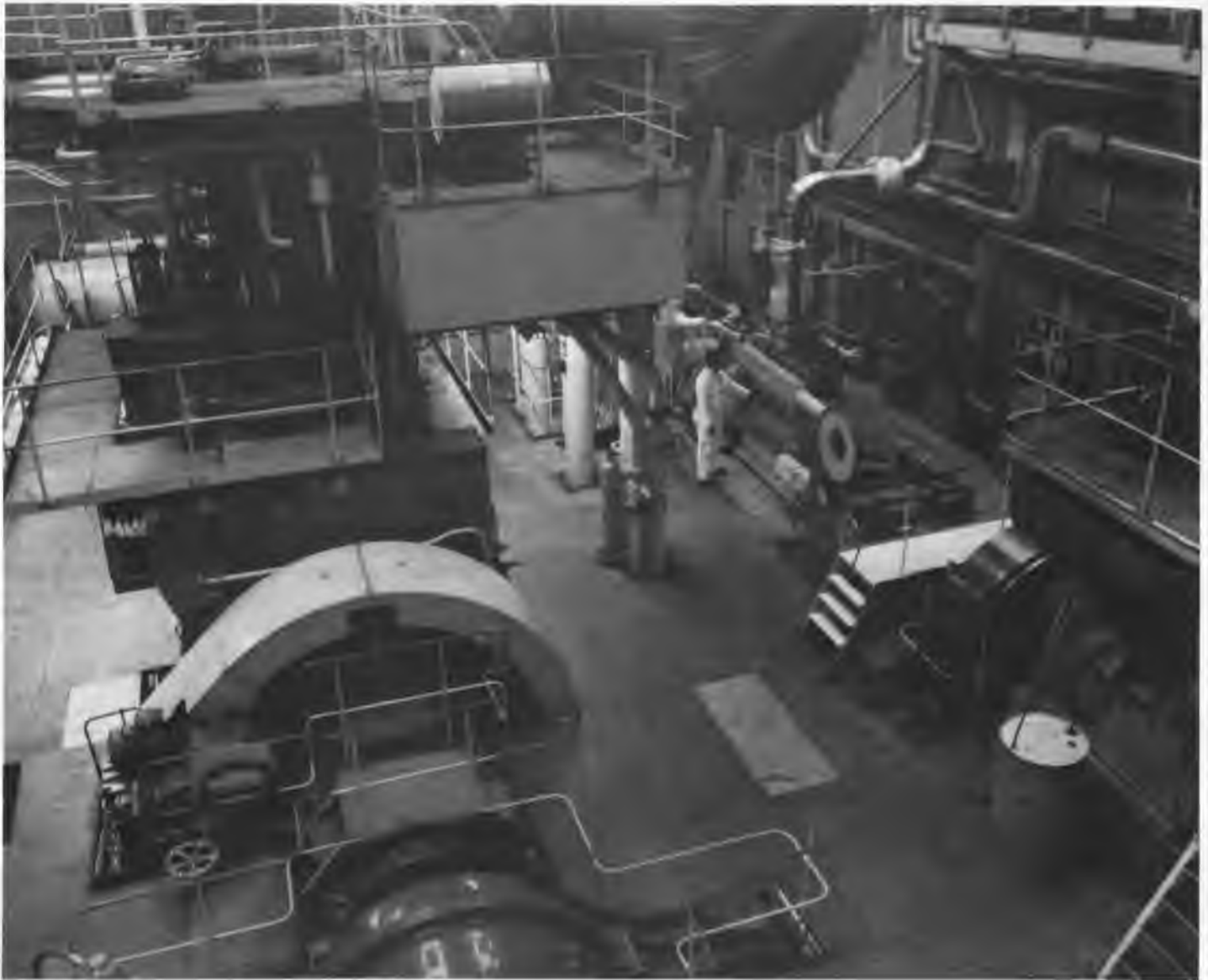
Fig. 2. Marine diesel testengines at KSLA. Left: Sulzer 2RNF 68M engine. Right front: Sulzer 1T48 engine. Right back MaK 1M282
