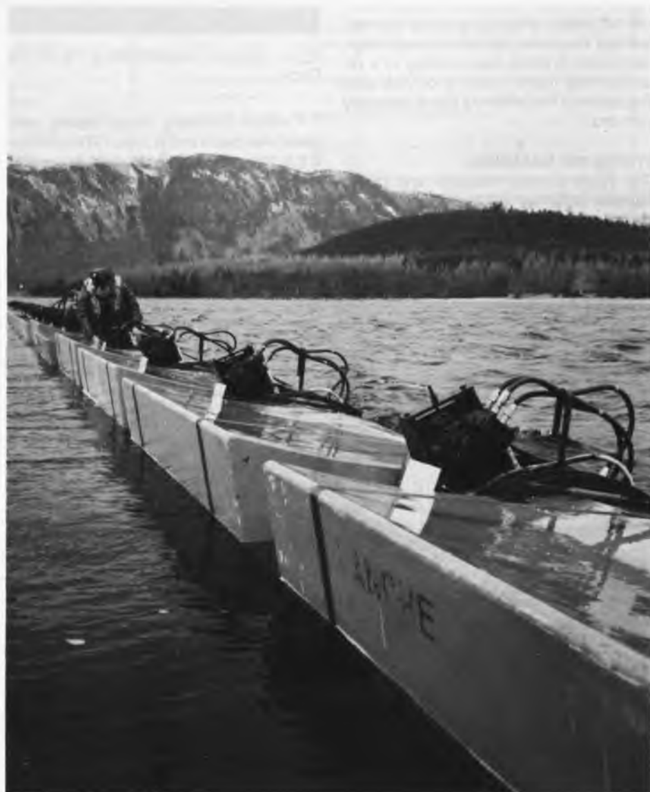
fig. 5. A 1/10 scale version of the Oscillating Vane tested on Loch Ness
